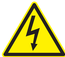
Electric Shock Hazard
